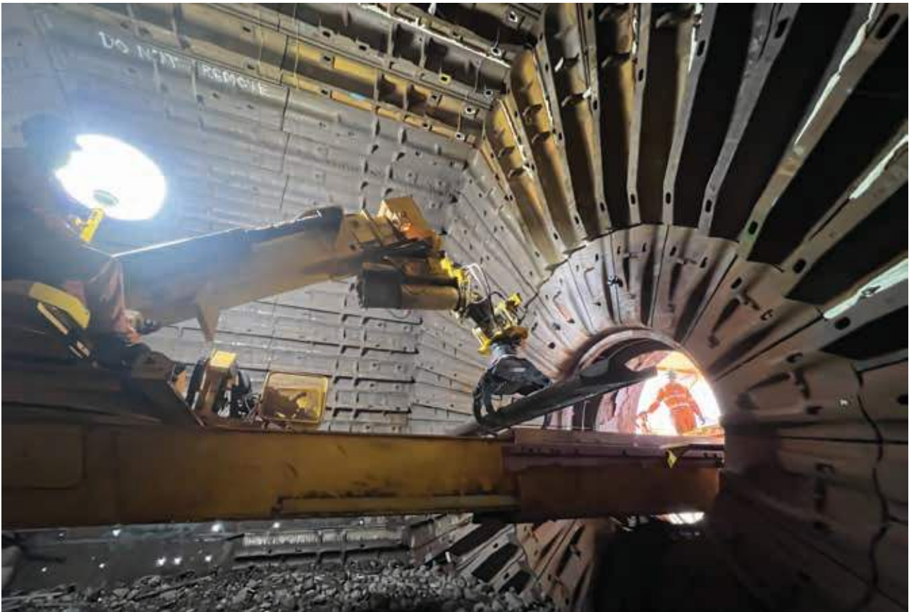
The RME Advanced Technology Mill Relining System relocates crew away from hazardous confined spaces during grinding mill maintenance. Many of its tools can be affordably retrofitted to existing RUSSELL Mill Relining Machines, ensuring widespread industry adoption.
