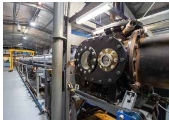
HypersonicLab: UniSQ's hypersonic wind tunnel facility investigates aerodynamics and heat transfer on aerospace vehicles.
